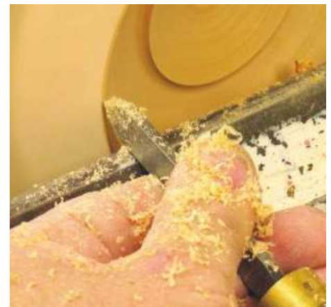
▲ Pic.27 Adding a little step with a freshly sharpened parting tool will add that little detail that breaks the transition between the upwards curve of the rim and the convex curve into the bowl – good to know!
